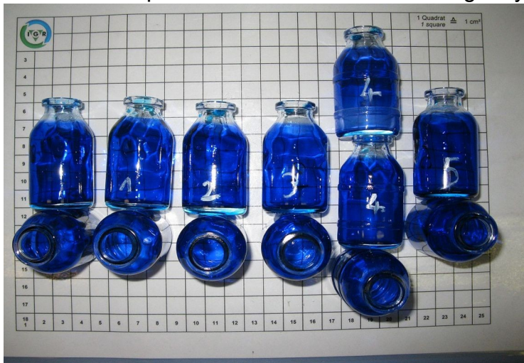
Abb. 1: Type III-bottles with corrosion visualized via methyl blue
